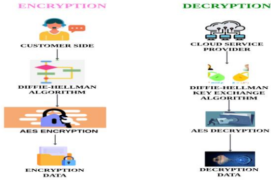
Figure 1: Cloud Data Security with Diffie-Hellman Key Exchange and AES Encryption.
